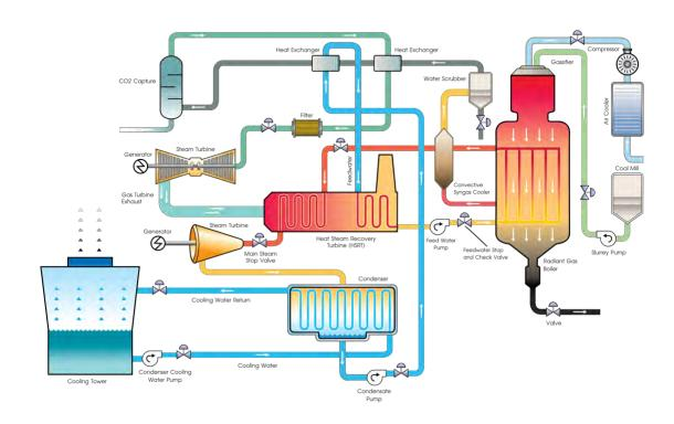
A combined cycle just means that the power plant "combines" or uses two plants so that they can recycle the heat generated by one plant for the other adjacent plant, thereby increasing the efficiency of electricity production.
